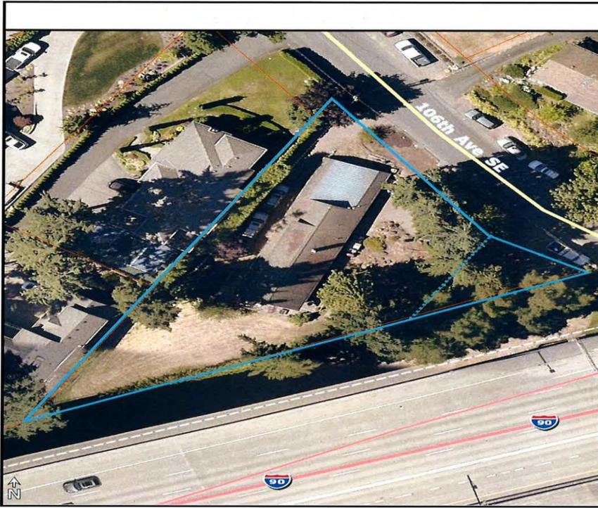
Bennett property boundary in blue. WTD needs a five foot permanent easement along the entire south property line parallel to I-90, and an an additional eight foot temporary construction easement along approximately a third of the south property line.
