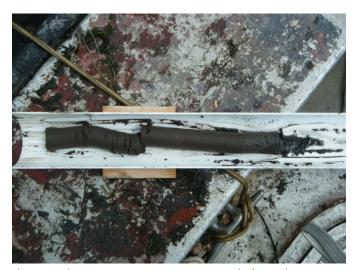
Photograph 10. Representative core sample (Sample 4A, shoreward of Lake Line). Top of core is at right.
