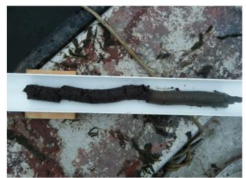
Photograph 10. Representative core sample (Sample 2B). Top of core is at right.
