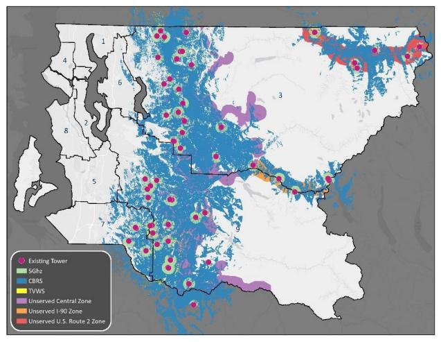
Almost all addresses that have 5 GHz coverage also have CBRS coverage. Although no more addresses are reached by adding 5 GHz than by just deploying CBRS, there may be some cases where CBRS capacity is at a maximum and 5 GHz could be deployed to offload some of the traffic.
