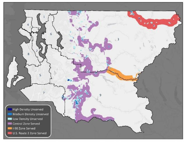
CTC determined 10 optimal locations for new towers based on their ability to reach most of the remaining addresses. However, we found that only six of the 10 locations were each able to cover more than five unserved addresses—which illustrates the difficulty of adding new towers that will cover a substantial number of addresses, and the low incremental value of these towers.
