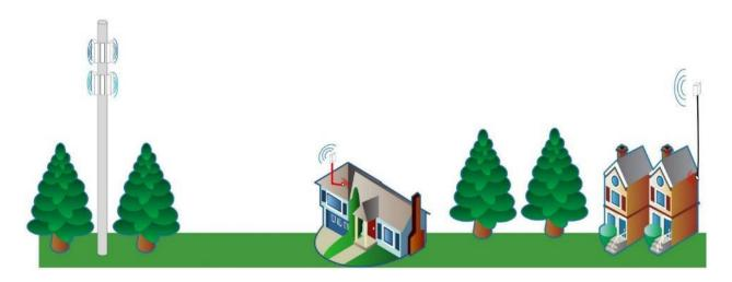
Figure 38: Example Fixed Wireless Network with Antennas on a Monopole and Customer Premises
