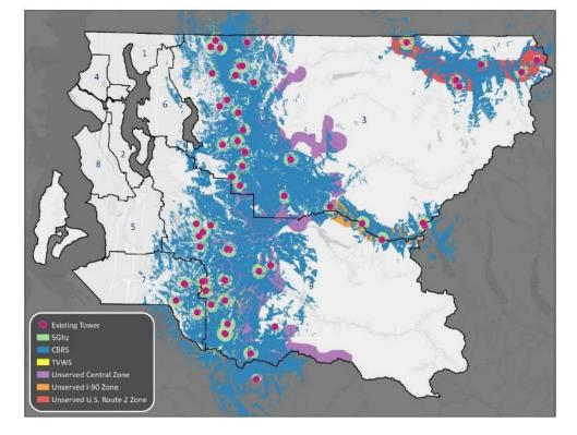
Figure 6: Fixed Wireless Coverage Using Public Safety Towers and Other Existing Towers
