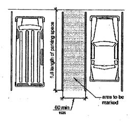
Locate accessible parking spaces on the shortest accessible route of travel to an accessible building entrance (where practical, not crossing traffic lanes).
