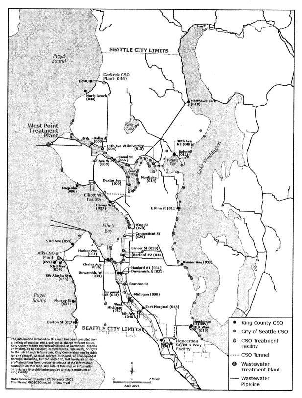
Figure 2-7. Combined Sewer Overflow (CSO) Locations
