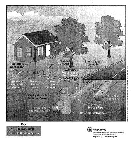
Figure 2-6. Sources of Infiltration and Inflow
