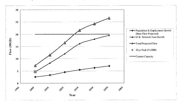
Figure 3-4. Example of Flow Projections Versus Existing Capacity in a Model Basin
