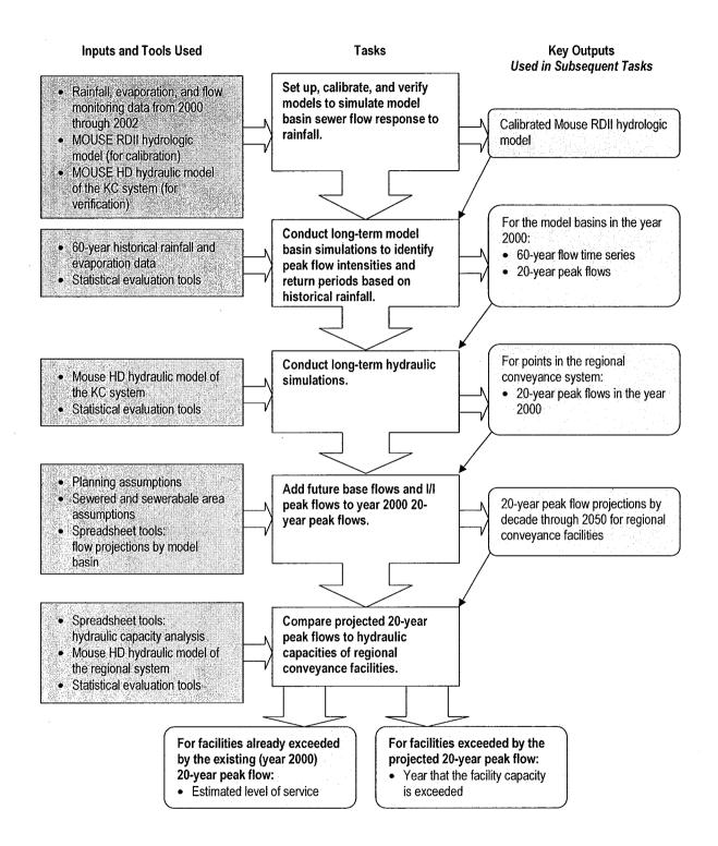
Figure 3-3. Process for Identifying Capacity Needs
