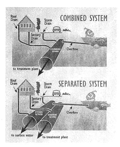
Figure 2-2. Combined and Separated Sewer Systems
