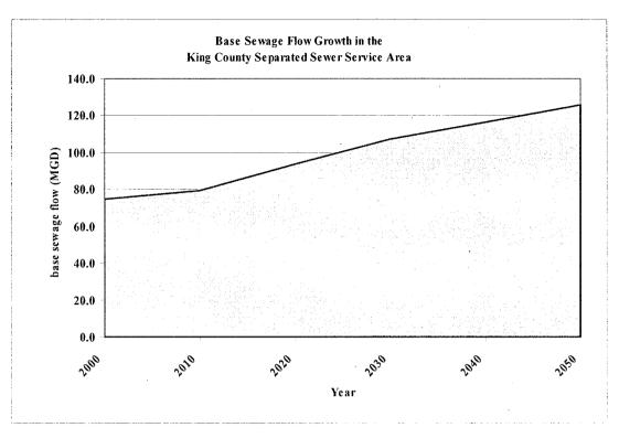
Figure 3-2. Projected Base Flow for the Regional Conveyance System (2000–2050)
