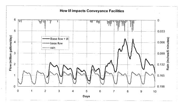
Figure 3-1. Typical Hydrograph Showing Impacts of I/I on Wastewater Flows
