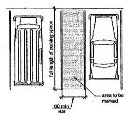
Locate accessible parking spaces on the shortest accessible route of travel to an accessible building entrance (where practical, not crossing traffic lanes).
