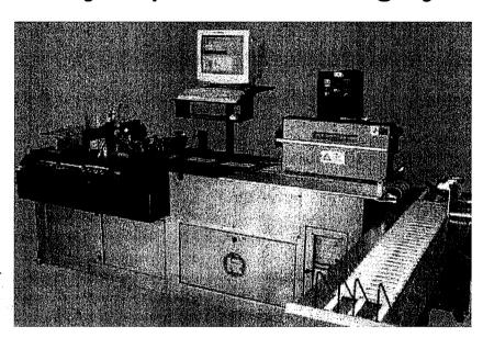
The Kirk-Rudy high speed duplex ink jet addressing system feeds each envelope individually, prints three inches of print, turns the envelope over and prints three inches on print on the reverse of the envelope.
