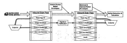
**Tracking and Audit Trail** - After the completed ballots are received (from mail or over the counter), they are processed through the Incoming Process on the Image Link Sorter using the same File-Based control file. Each ballot is processed against the same file and record as when it was processed for outgoing. This continuity of data tracking allows for a complete integrity solution therefore enabling automated reconciliation and real-time status and management reporting.
