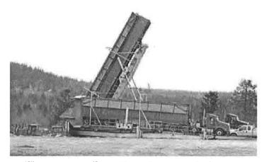
Landfill tippers are an efficient way to empty transfer trailers
