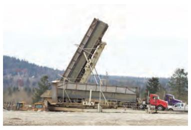
Landfill tippers are an efficient way to empty transfer trailers
