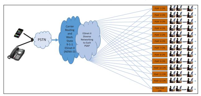
Figure 3 - ESInet-II Networking at Completion of Migration - King County PSAPs Still on Existing 911 Systems
