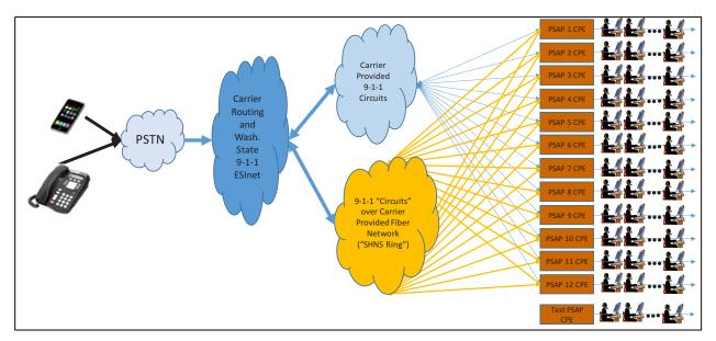
Figure 1 - Current Call Routing and Transport for King County PSAPs
