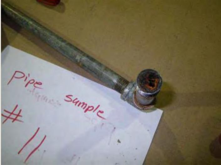
**Figure 4 Pipe Sample from Courthouse domestic water system**
