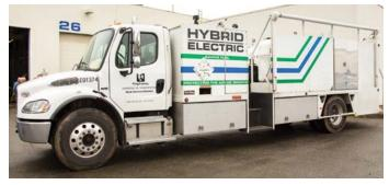
This hybrid service truck supports field preventive maintenance on fleet vehicles and equipment. The truck uses the hybrid battery to operate the air compressor and 12 volt/110 volt electrical systems making it unnecessary to run the engine when carrying out service operations.
