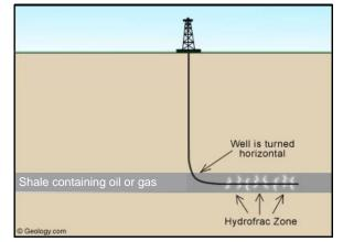
Horizontal drilling involves creating an initial vertical bore of up to several thousand feet, then turning the drill and continuing horizontally for up to several miles.
