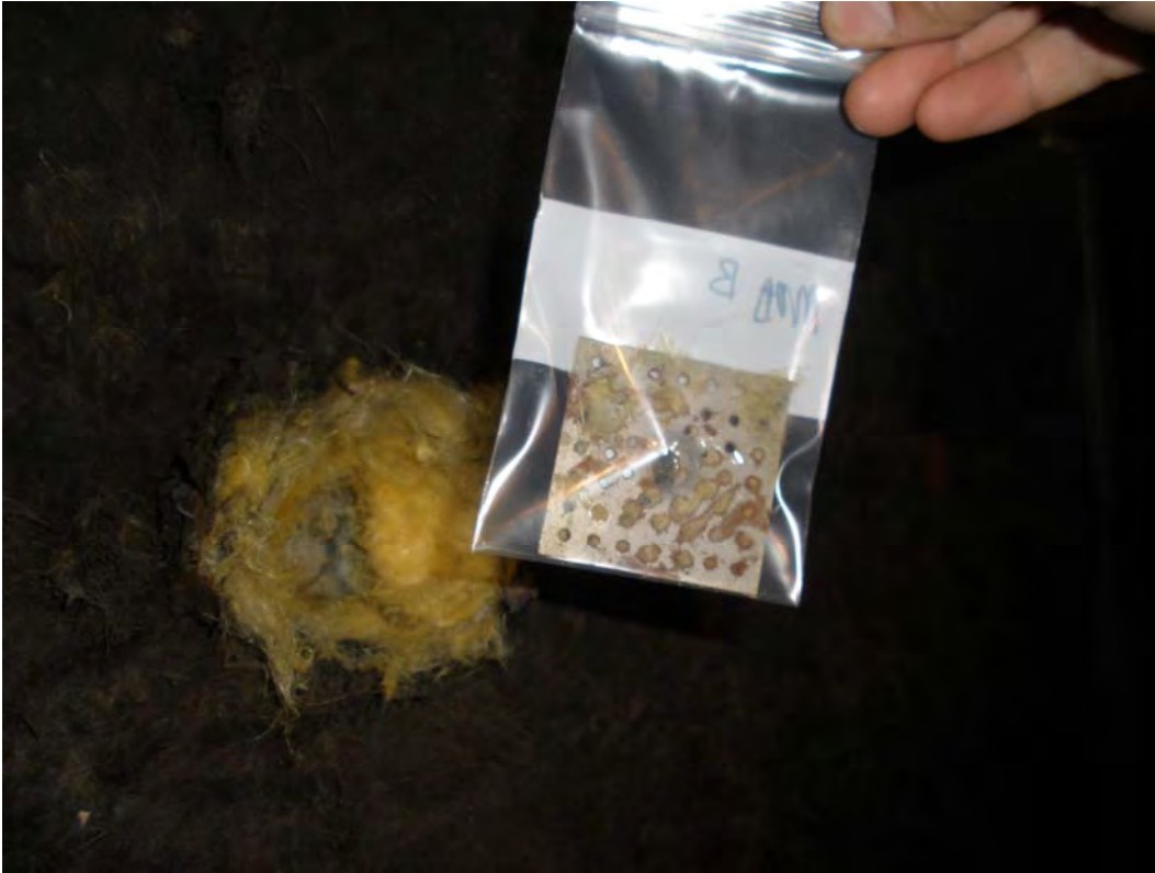
Photo 23. ACM stick pin adhesive on mechanical room door-Alder Wing
