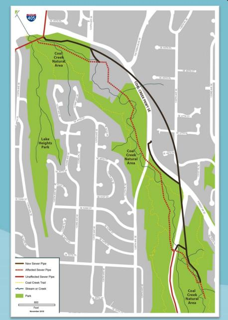
Increase conveyance capacity of the Coal Creek Interceptor from 7-10 mgd to 11-19 mgd (flow depends on location).
