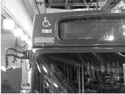
The photograph above shows an acceptable installation on a New Flyer DE60LF by King County personnel. The tag/reflector assembly should butt up against the bottom of the clearance light for optimal performance.
