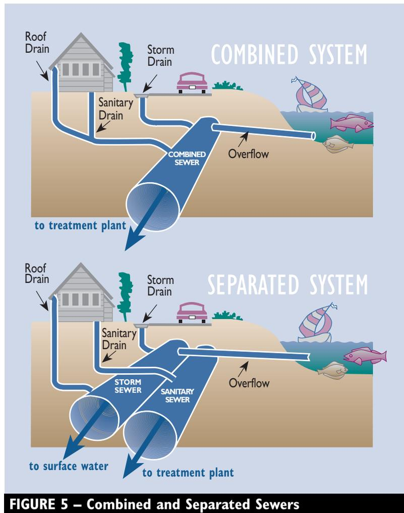
**FIGURE 5 – Combined and Separated Sewers**
