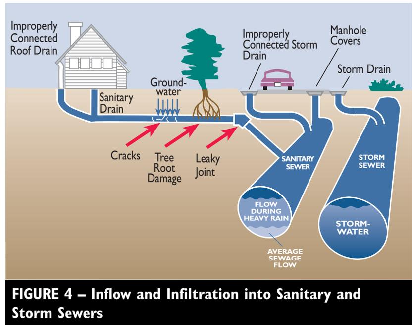
**FIGURE 4 – Inflow and Infiltration into Sanitary and Storm Sewers**
