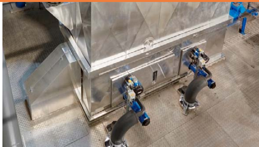
Fluid Bed with direct injection nozzles in foreground
