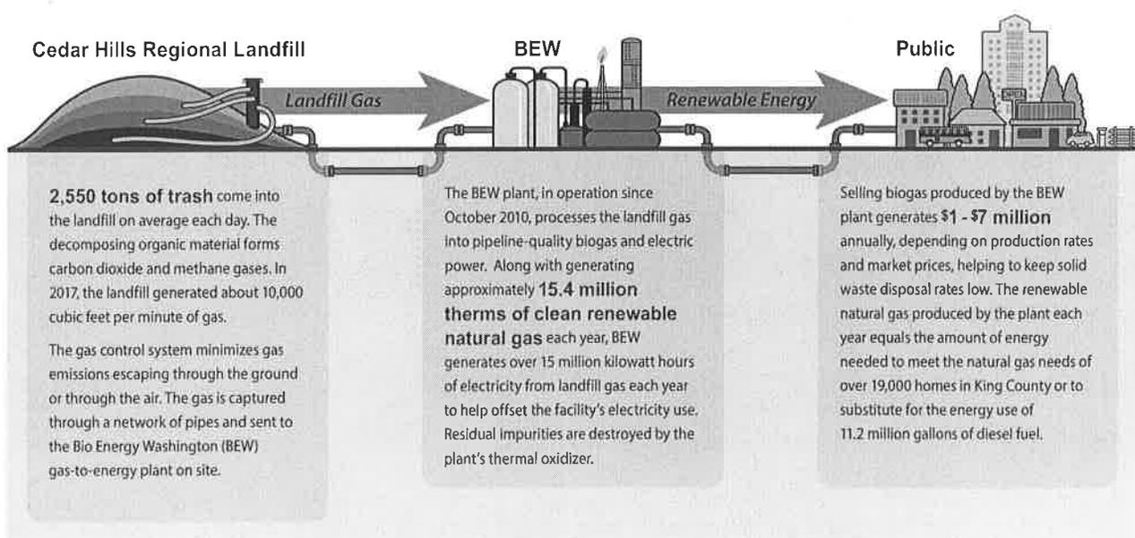
The gas collected from the landfill is sent to the Bio Energy Washington plant to be processed into pipeline quality gas
