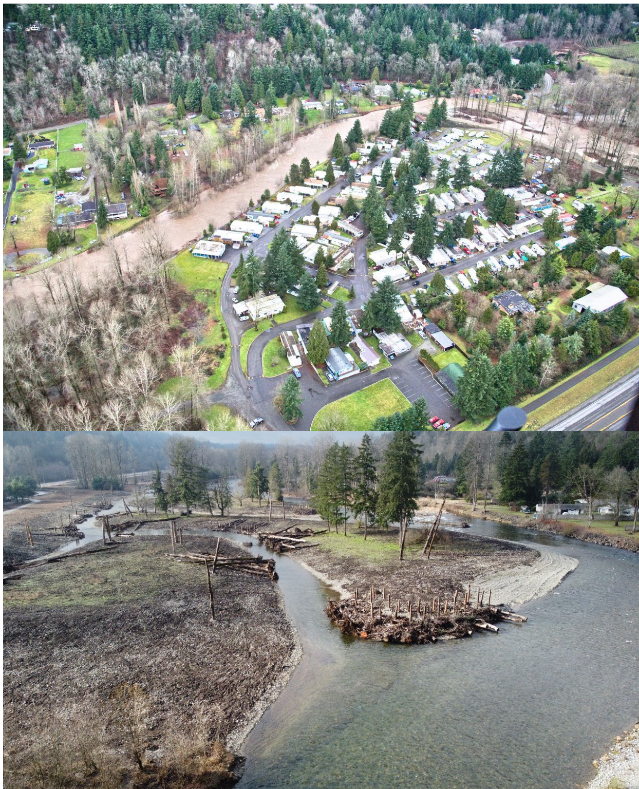
Before (top) and after (bottom): Riverbend Manufactured Home Community on Cedar River before acquisitions (2009, looking upstream) and the same site after Riverbend Levee Setback and Floodplain Restoration project (2023, looking downstream)
