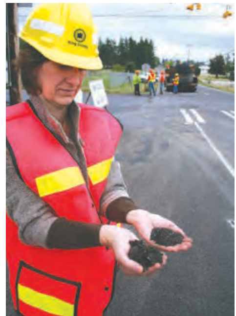
Developing markets for asphalt shingles has been one focus of the LinkUp program. Shown here are asphalt shingles used in paving roads
