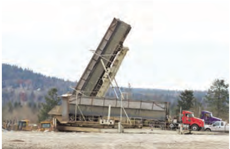
Landfill tipplers are an efficient way to empty transfer trailers
