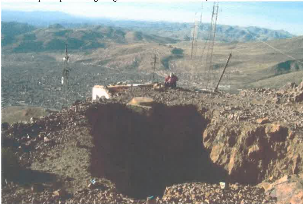
3/26/'19 Photo 5: MINE COLLAPSE UNDER MOUNTAIN. ISSUE OF SUBSIDENCE (source: Wikipedia photos in geological feature "Subsidence").
