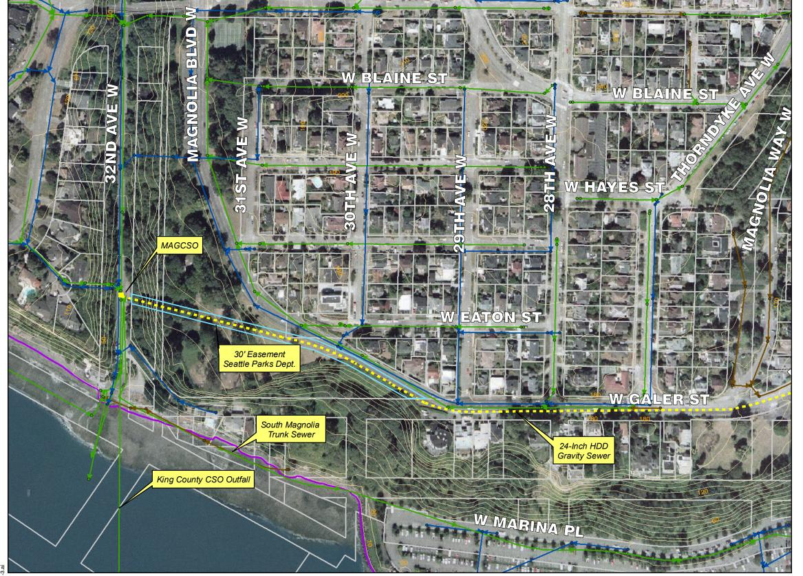
A 30-foot wide subterranean easement for a conveyance pipe to be installed by directional drilling underneath seven of the following potential parcels:
