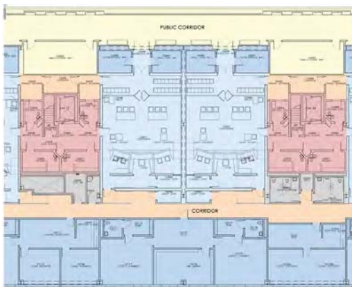
The court wing includes five courtrooms, hearing rooms, and self help areas with extensive administrative and public support areas. To facilitate a more calming, effective and therapeutic juvenile justice system, related justice agencies are collocated with the courts.
