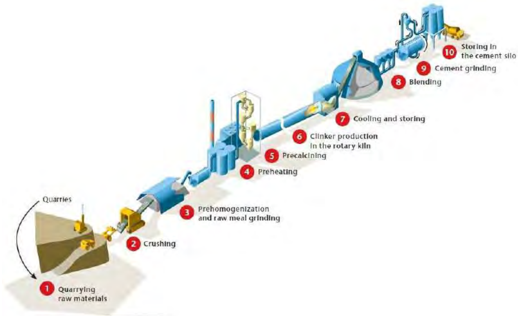
Figure A.1. Steps in the cement production process using the new suspension preheater and precalciner kiln (WBCSD/IEA 2009a)
