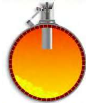
Figure 33. Cadence's mid-kiln fuel injector technology (Cadence 2012a).
