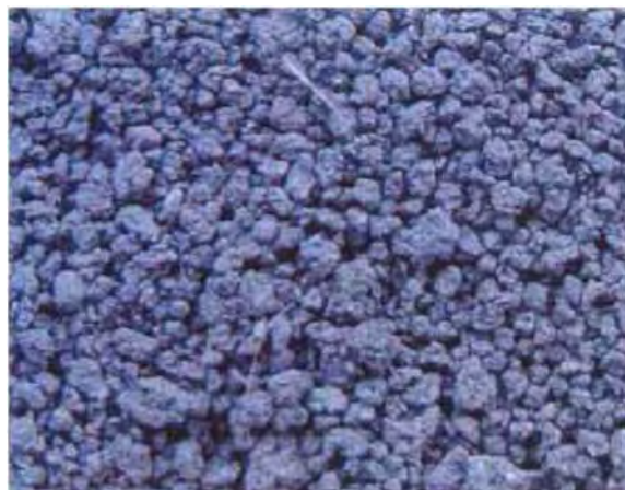
Dried granules from Fluid Bed Dryer
