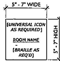
Non-code required panel signs (or fixed signs for dedicated use rooms), such as "Computer Room," "Storage," or "Parts Room" can be sized accordingly. This is also applicable to Special Signs, such as "Upstairs to Administration," to assist with wayfinding.
