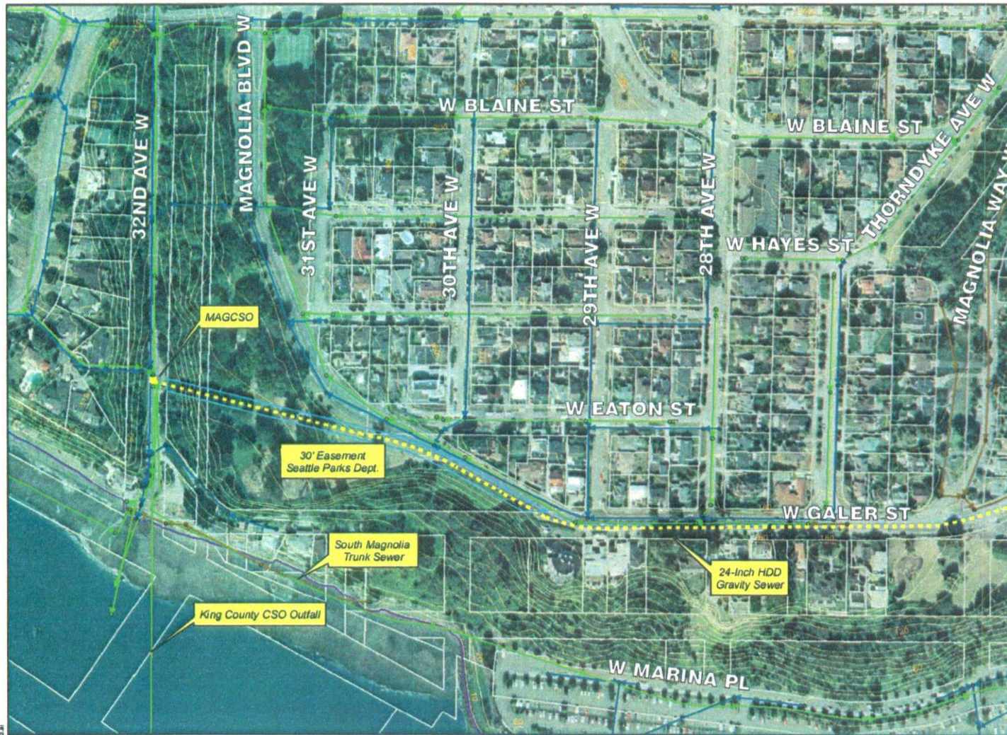
FIGURE 1.3.3A A 30-foot wide subterranean easement for a conveyance pipe to be installed by directional drilling underneath seven of the following potential parcels:
