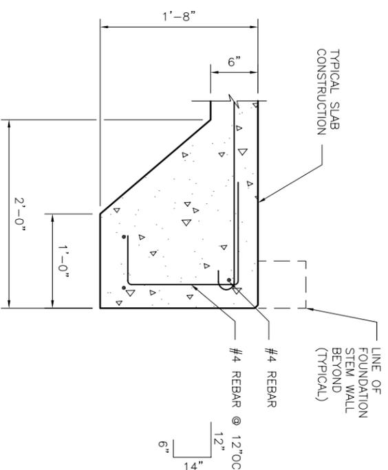
**FOUNDATION AT DOOR OPENING SECTION B**
