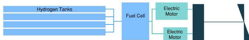
Future Propulsion Configuration - Fuel Cell Option (one per hull)
