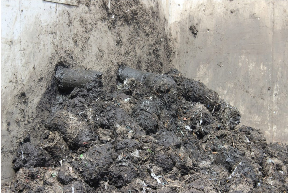
Figure 2-3. Fitec, Rothmuhle biogas plant in Germany: extruded solid fraction from BioSqueeze unit
