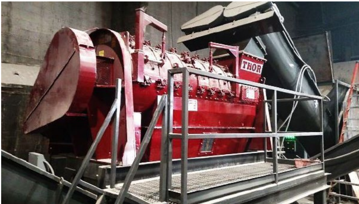
Figure 2-6. Scott Thor organics de-packager (aka turbo separator)
