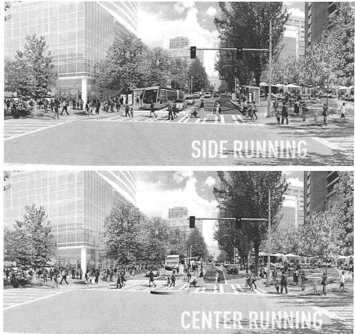
FIGURE 4-2. SIDE AND CENTER RUNNING CROSS SECTIONS
