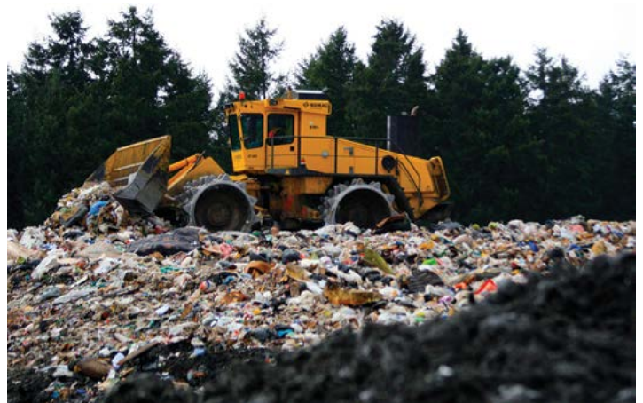
Compacting garbage at the Cedar Hills Regional Landfill
