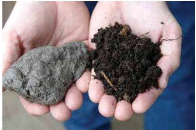
The difference between heavily compacted and healthy amended soil from the same site is very apparent. Source: Dirt Doctor .
