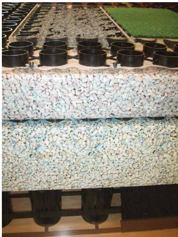
This mock up shows a typical cross section of engineered subsurface that contributes to permeable surfaces. Source: O'Brien & Company.
