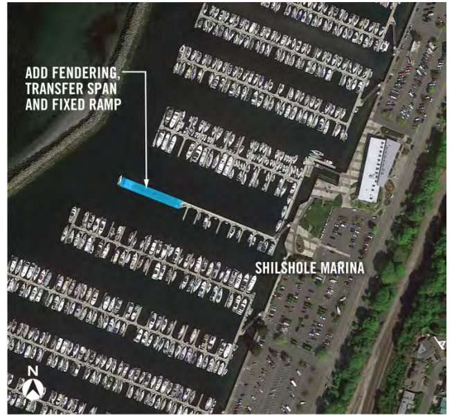
Figure 13: Ballard Proposed Infrastructure Improvements
