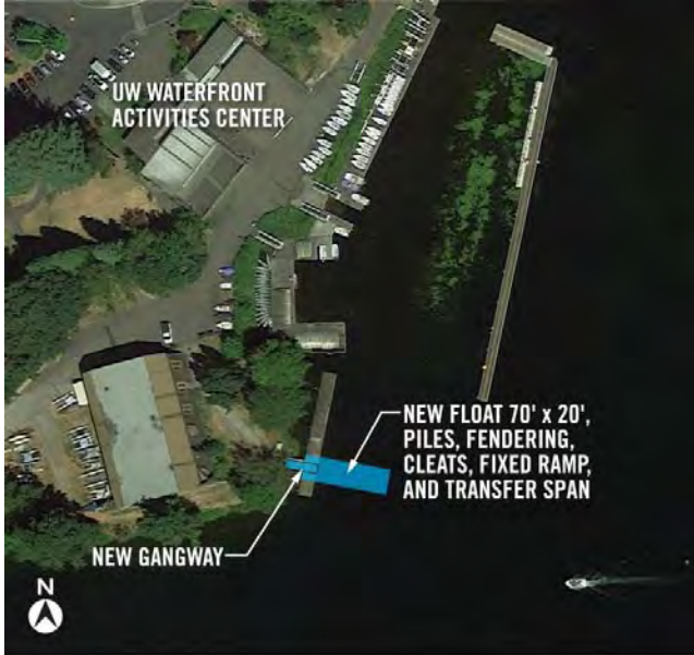
Figure 10: UW WAC Proposed Infrastructure Improvements
