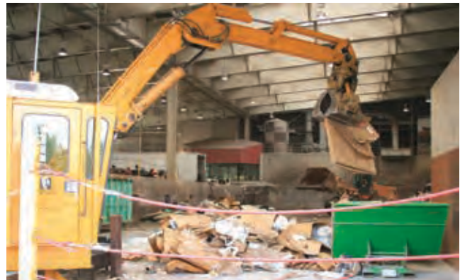
A Transfer Station Operator recovers cardboard from a mixed load of solid waste
