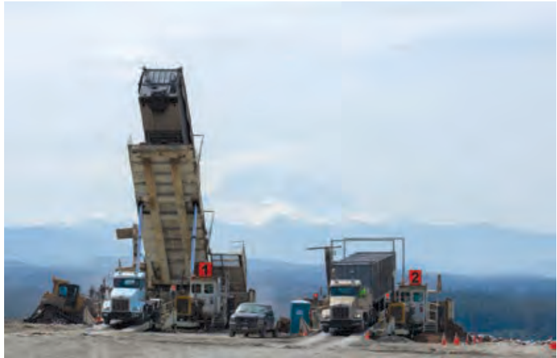
Tippers empty trailers more efficiently
